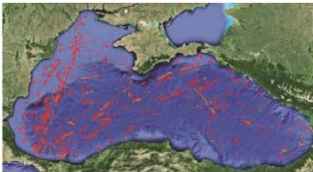
. Map of oily ship discharges to the Black Sea, detected as a result of the analysis of satellite radar data in 2009-2011 [15].
