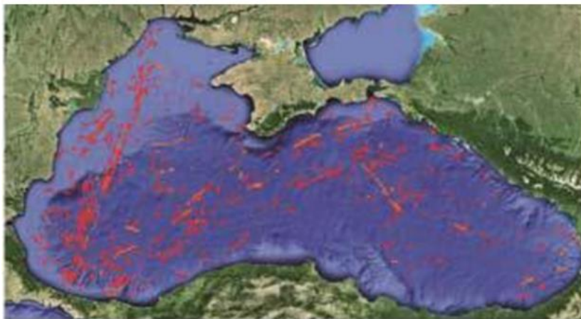
Fig.15 Map of oily ship discharges to the Black Sea, detected as a result of the analysis of satellite radar data in 2009-2011.
