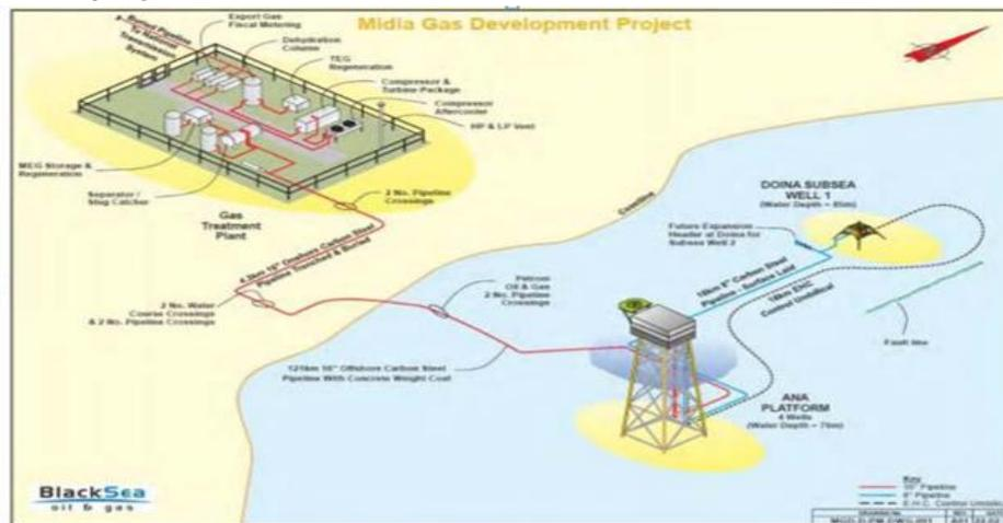
**Fig.2 Schematic Concept for Midia Gas Development**
